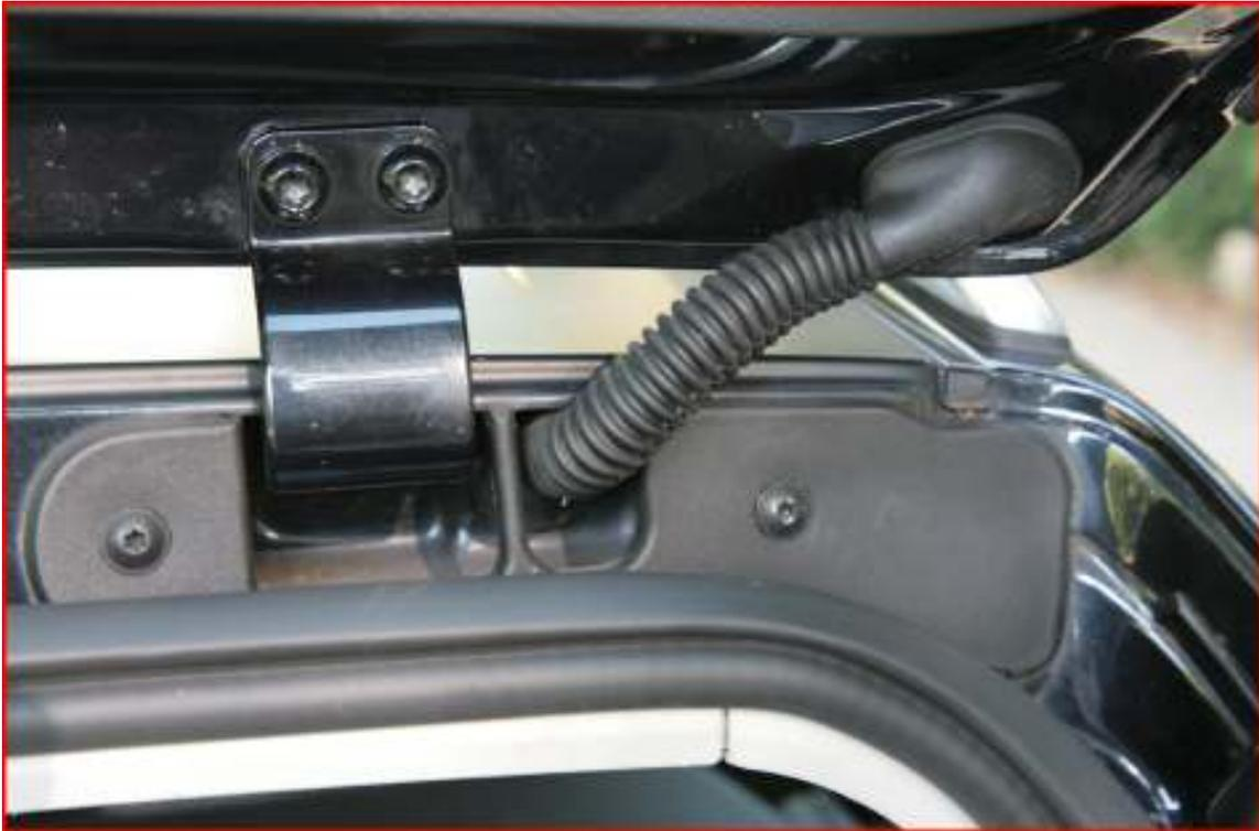
You will want to remove the plastic cover (two torx screws) to give yourself more room to work (note that I've also pulled the accordion hose from the hatch):
