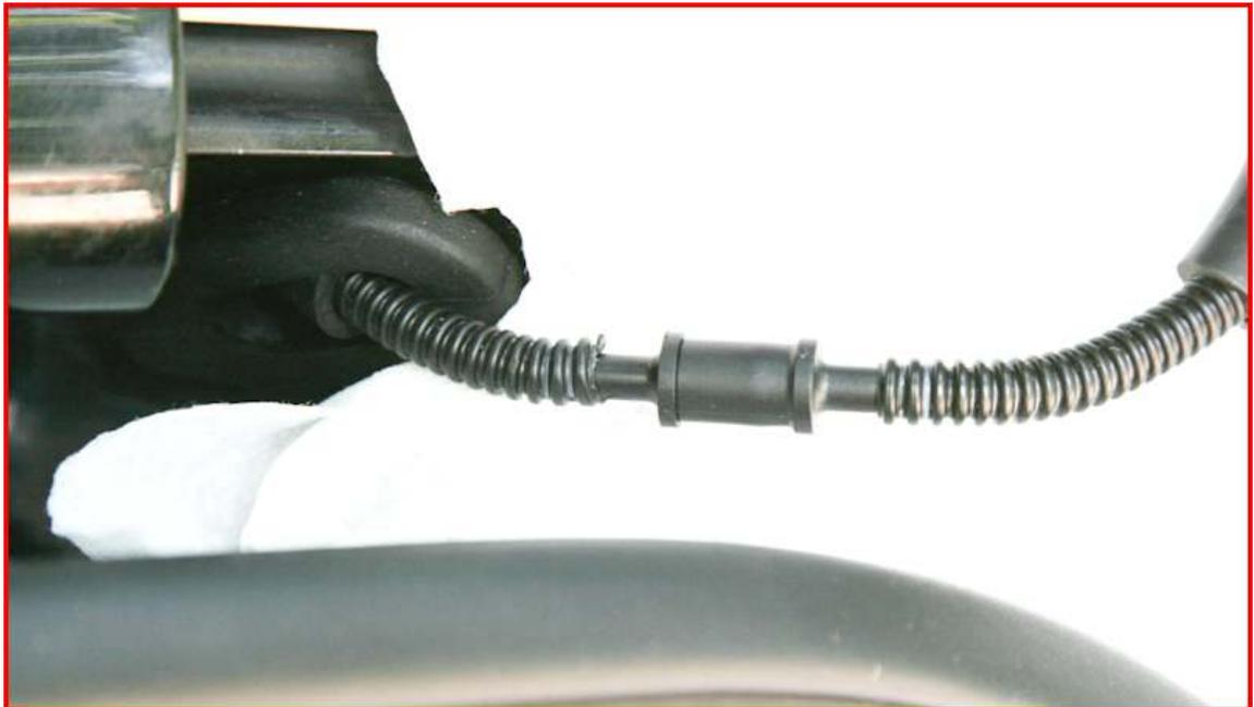
10. Remove thread from washer fluid line ends
