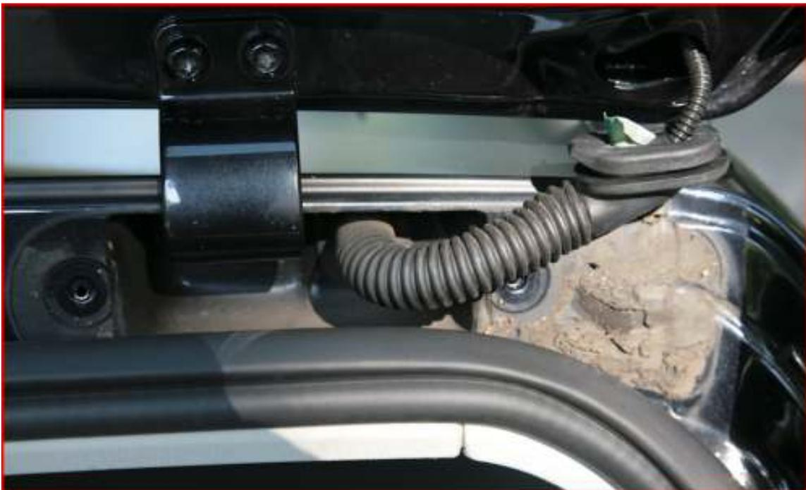
The hose runs all the way through the car and exits at the right rear hatch hinge. Gently pull the rubber accordion hose off the hatch as I have in the picture
