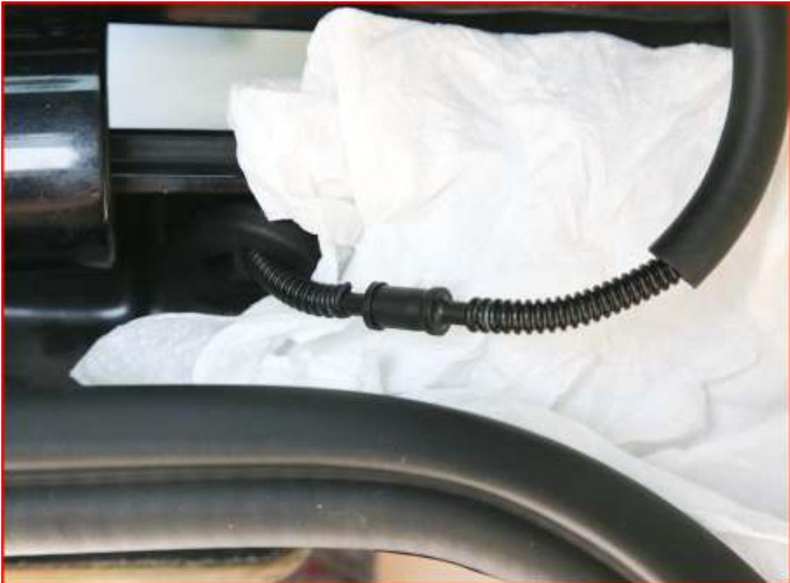
If, however, your plastic hose broke closer to the roof (like mine did), you're in for a bit more work. Why? The answer is simple: you can't repair the plastic hose without cutting open or removing the accordion hose, and you can't squeeze it / compress it enough to keep it out of the way while you repair the plastic hose.
