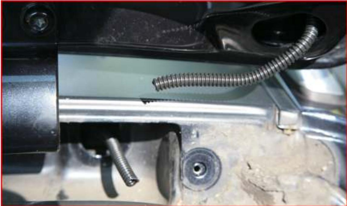
4. Note where the break in the washer fluid line (inner layer) is, and eyeball where it corresponds to on the black rubber hose (middle layer). This hose, when properly placed over the washer fluid line, will be roughly 40% in the hatch, and 60% in the car. Cut the rubber hose to correspond to where the break is.
